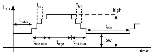
**Figure 4. LM2755 LED Timing Control**
