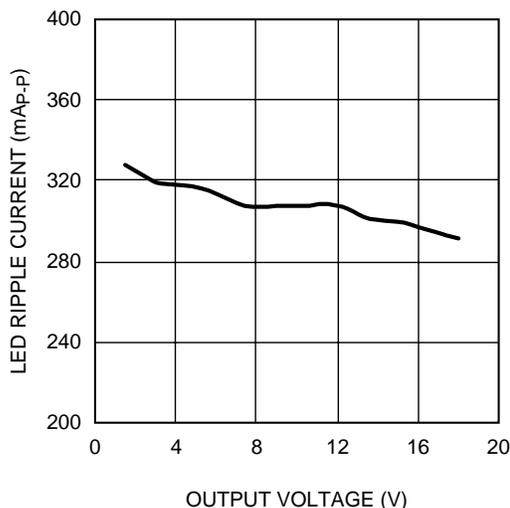
Figure 2. Ripple Current vs. Output Voltage
