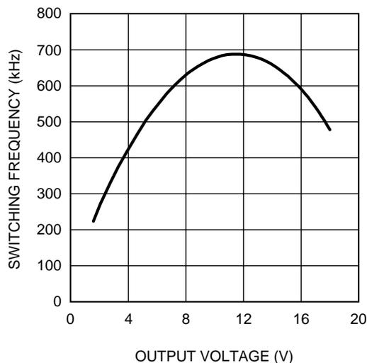
Figure 3. Switching Frequency vs. Output Voltage
