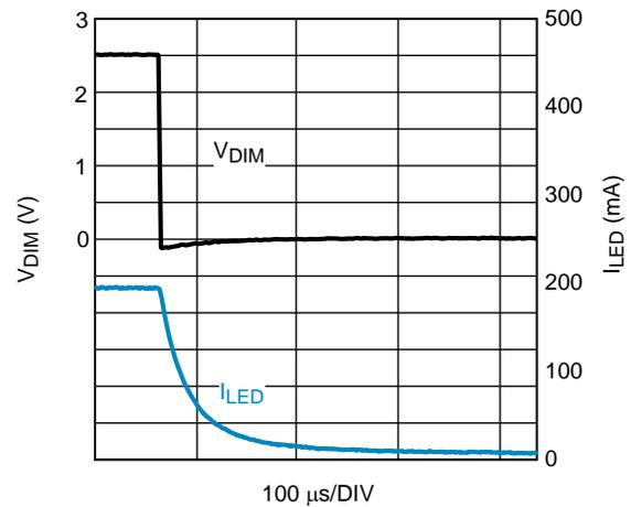
Figure 7. 500Hz PWM Dimming (Falling Edge), 50% Duty Cycle,  $V_{IN} = 3.3 \text{ V}$
