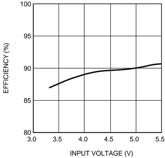
Figure 4. Efficiency vs. Input Voltage,  $I_{LED} = 190 \text{ mA}$
