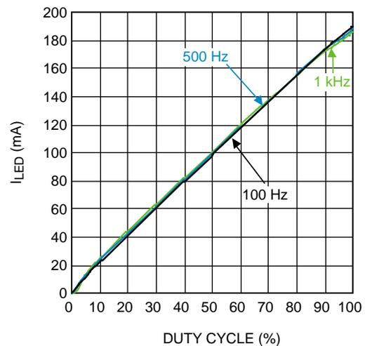
Figure 3. PWM Dimming,  $V_{IN} = 5.5\text{ V}$
