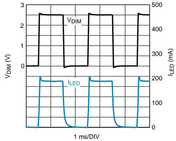
Figure 5. 500Hz PWM Dimming, 50% Duty Cycle,  $V_{IN} = 3.3 \text{ V}$
