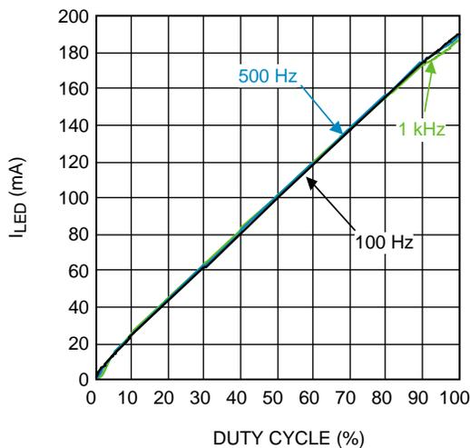
Figure 2. PWM Dimming,  $V_{IN} = 3.3\text{ V}$
