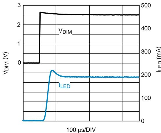
Figure 6. 500Hz PWM Dimming (Rising Edge), 50% Duty Cycle,  $V_{IN} = 3.3 \text{ V}$
