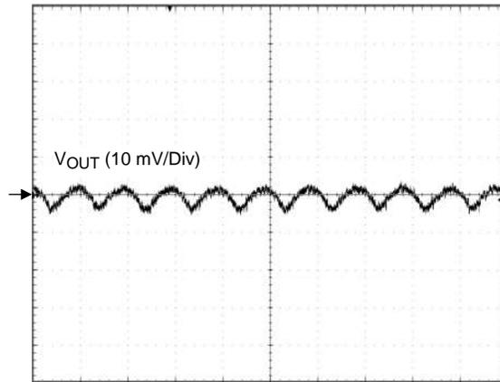
**Figure 4. Output Ripple Waveform (1 μs/DIV)**
