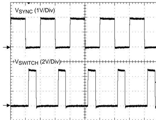
**Figure 5. Primary Switch Node Waveform (1 μs/DIV)**
