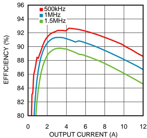
Figure 2. Conversion Efficiency Versus Output Current
