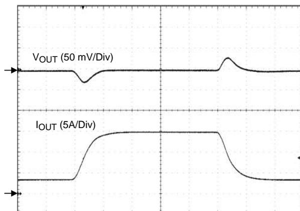
Figure 6.  $V_{OUT}$  Transient Response (40  $\mu$ s/DIV)
