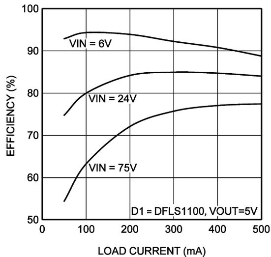
Figure 5. Efficiency at 200 kHz
