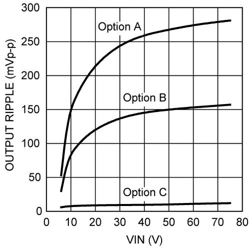
Figure 7. Output Voltage Ripple
