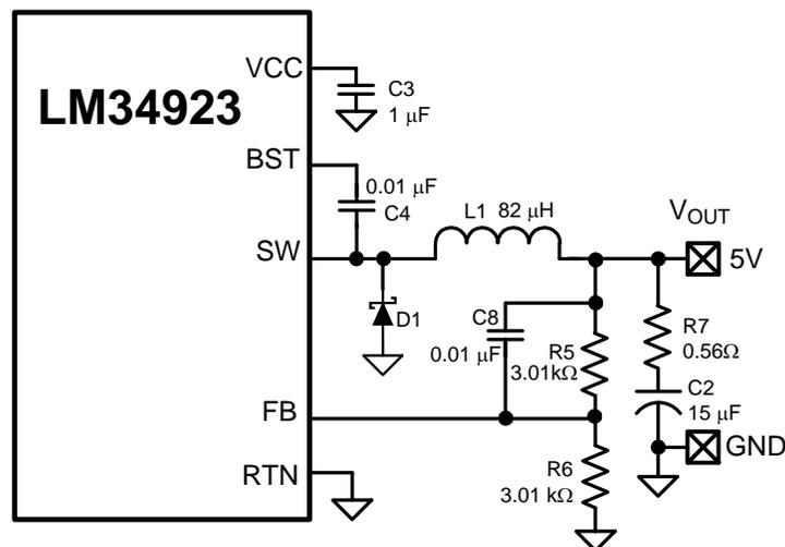
Figure 3. Reduced Ripple Configuration
