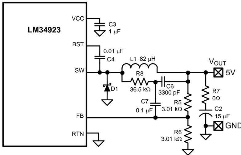
Figure 4. Minimum Output Ripple Configuration
