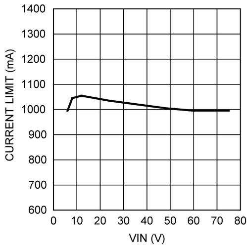
Figure 9. Current Limit vs. Input Voltage
