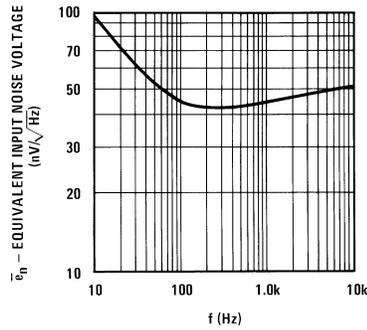
FIGURE 5. Noise Measurements
