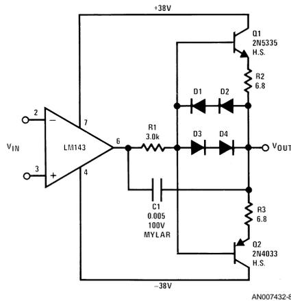
Heat sink is a Thermalloy No. 2230-5 or equivalent. All diodes are 1N914. All resistors are 1/2W, 10%.
