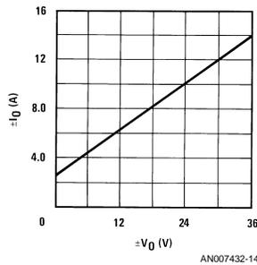
FIGURE 14. Output Current Limiting as a Function of Output Voltage
