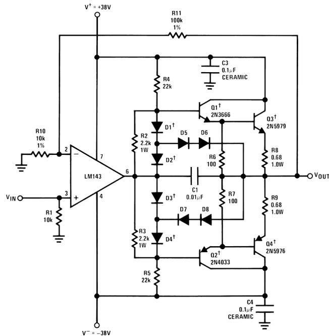
†Put on common heat sink, Thermalloy 6006B or equivalent.
