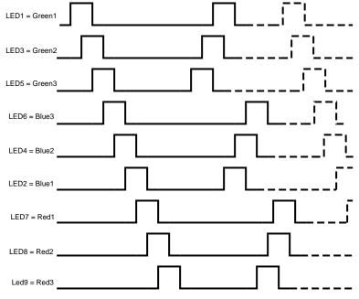
Sequence for Mux\_inc, Mux\_dec and Mux\_set Examples
