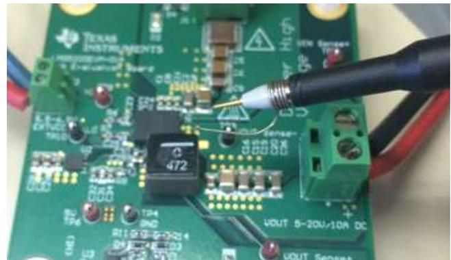
**Figure 6. Small GND Loop**
