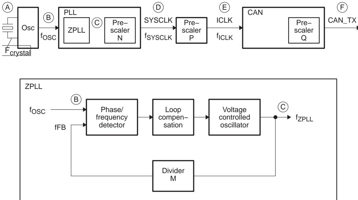
**Figure 1. Dependency of PLL Clock Jitter on the CAN Bit Timing**
