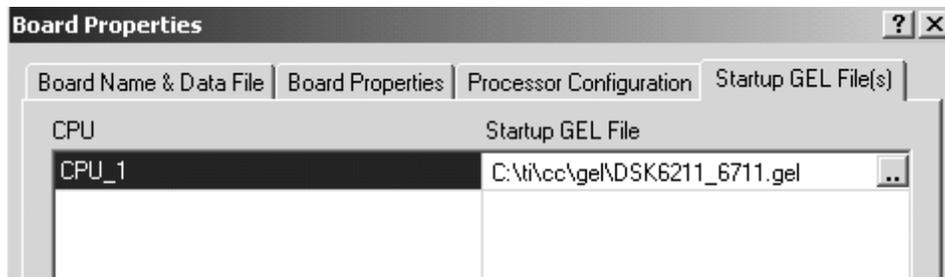
If you use simulation, select “C6711 Sim Ltl Endian.” The cycle counts obtained from simulation might not be accurate, especially with off-chip memory accesses.
