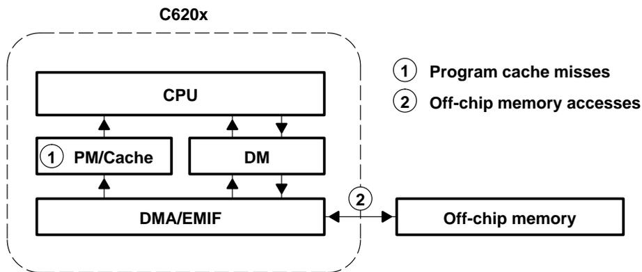
**Figure 1. C620x Memory Hierarchy and Potential Overhead**
