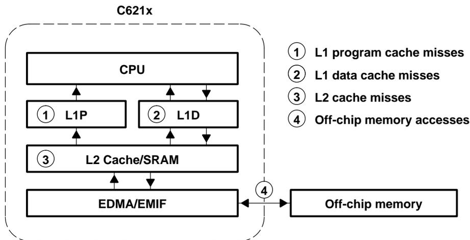
**Figure 2. C621x Memory Hierarchy and Potential Overhead**
