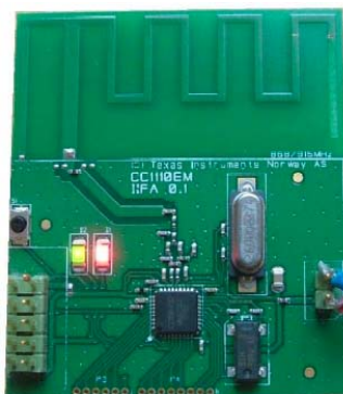
Figure 28. Inverted-F Antenna EM board for 868/915/955 MHz
