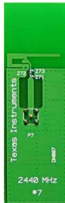
Figure 22. CC-Antenna-DK Board 7 - Inverted-F Antenna
