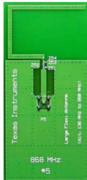
Figure 29. CC-Antenna-DK Board 5 - Loaded Stub Antenna (Large) for 868/915/955 MHz
