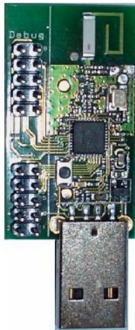
Figure 34. Chip Antenna from Johanson Technology for 868/915/955 MHz
