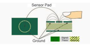
Figure 1. Capacitive Sensing Principle
