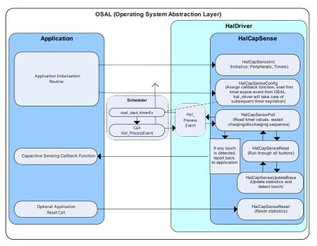
Figure 6. Capacitive Sensing Integration Architecture
