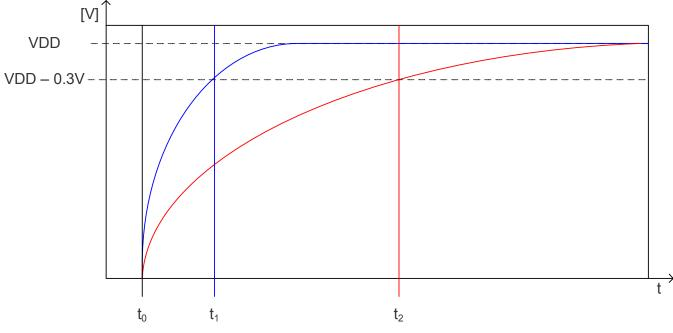
Figure 4. Rise Time With (t<sub>2</sub>) and Without (t<sub>1</sub>) Touch
