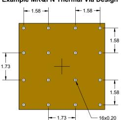
Example Via Layout Design Via layout may vary depending on layout constraints (Note D, F above)
