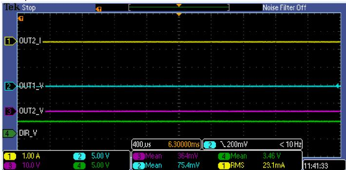
Section 4: Output Voltage, Output Current, and Direction Voltage for 50% duty Cycle
