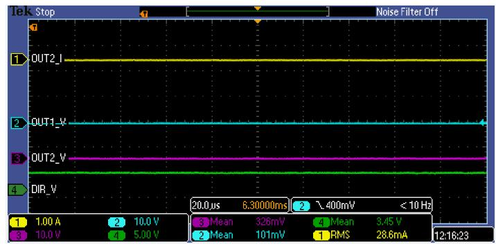
Section 5: Output Voltage, Output Current, and Direction Voltage for 20% duty Cycle
