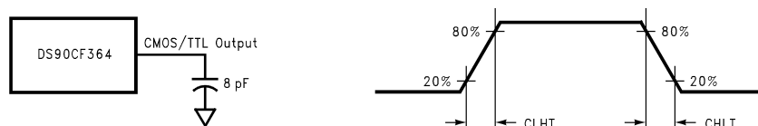
Figure 7. DS90CF364 (Receiver) CMOS/TTL Output Load and Transition Times
