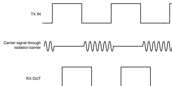
**Figure 12. On-Off Keying (OOK) Based Modulation Scheme**
