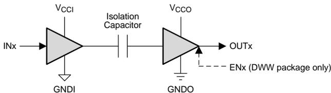
(1) V<sub>CCI</sub> and GNDI are supply and ground connections respectively for the input channels.
