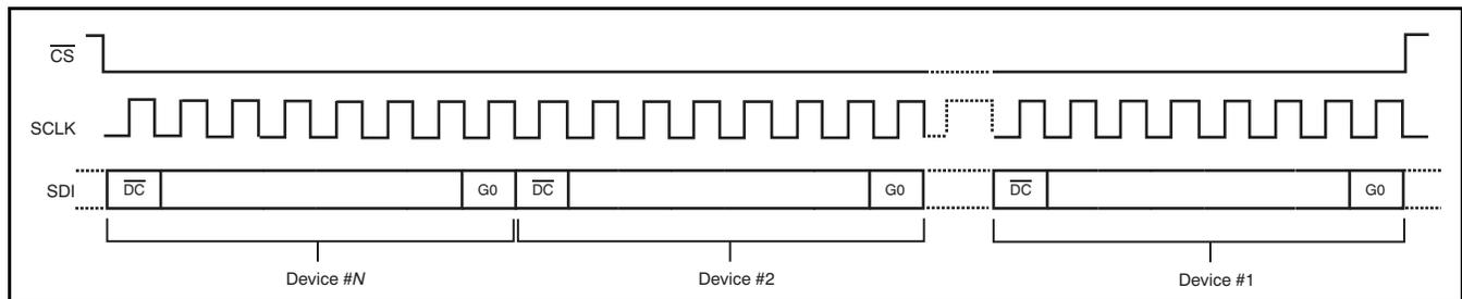
Figure 12. Serial Port Operation for Daisy-Chain Operation
