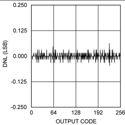
Figure 5. Dnl  $F_{\text{SCLK}} = 20 \text{ MHz}$
