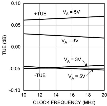
Figure 9. Total Unadjusted Error vs Clock Frequency
