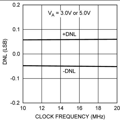
Figure 7. Dnl vs Clock Frequency
