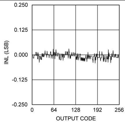
Figure 6. Inl  $F_{\text{SCLK}} = 20 \text{ MHz}$
