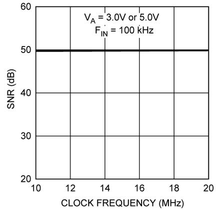
Figure 10. SNR vs Clock Frequency
