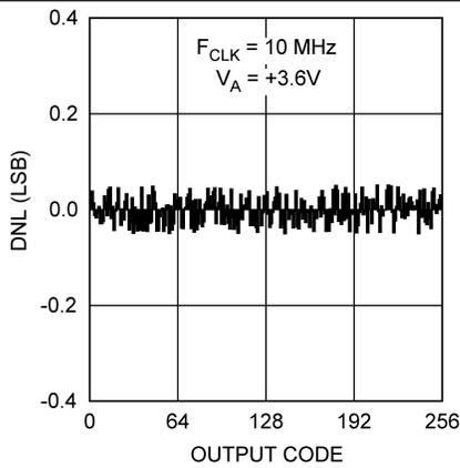
Figure 3. Dnl  $F_{\text{SCLK}} = 10 \text{ MHz}$
