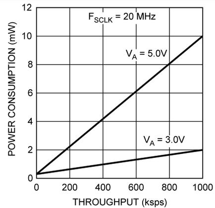
**Figure 16. Power Consumption vs. Throughput,  $F_{\text{SCLK}} = 20 \text{ MHz}$**
