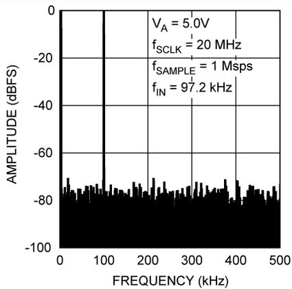
**Figure 15. Spectral Response,  $V_A = 5\text{v}$   $F_{\text{SCLK}} = 20 \text{ MHz}$**
