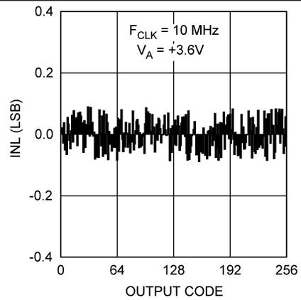
Figure 4. Inl  $F_{\text{SCLK}} = 10 \text{ MHz}$
