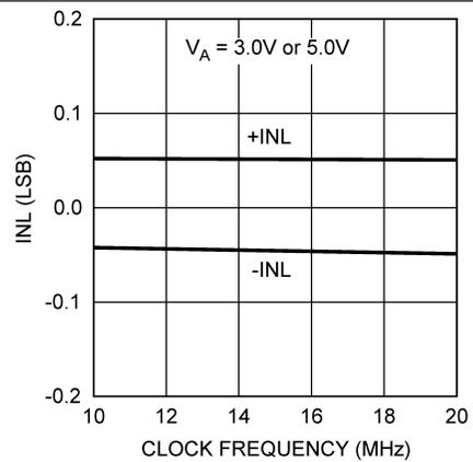
Figure 8. Inl vs Clock Frequency
