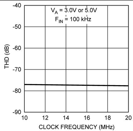
Figure 12. Thd vs. Clock Frequency
