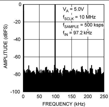
Figure 14. Spectral Response,  $V_A = 5\text{v}$   $F_{\text{SCLK}} = 10 \text{ MHz}$
