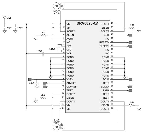
Figure 14. Typical Application Schematic
