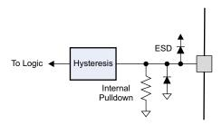
Figure 1. Logic Inputs
