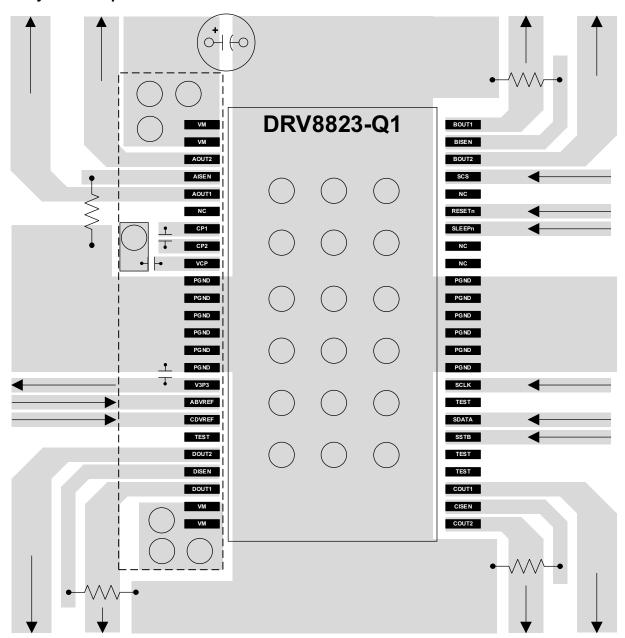
Figure 20. Typical Layout of DRV8823-Q1
