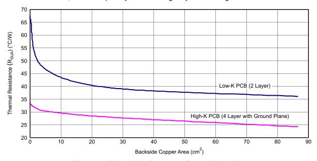
Figure 21. Thermal Resistance vs Copper Plane Area
