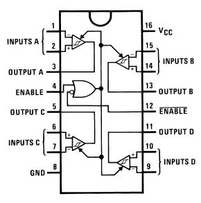
Figure 1. CDIP and CLGA Packages-Top View See Package Numbers NFE0016A, NAC0016A, or NAD0016A
