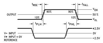
Figure 19. Propagation Delay
