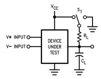
$C_{\text{L}}$  includes load and test jig capacitance.
