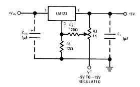
Figure 15. Trimming Output to 5V
