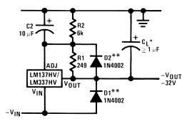
\*When C<sub>L</sub> is larger than 20 µF, D1 protects the LM137HV in case the input supply is shorted
