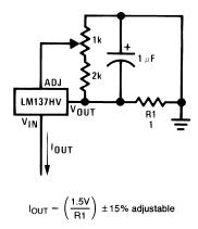
Figure 8. Adjustable Current Regulator
