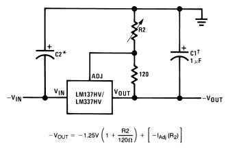
$^\dagger$ C1 = 1  $\mu$ F solid tantalum or 10  $\mu$ F aluminum electrolytic required for stability. Output capacitors in the range of 1  $\mu$ F to 1000 µF of aluminum or tantalum electrolytic are commonly used to provide improved output impedance and rejection of transients.
