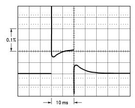
$$\begin{split} LM137HV, \ V_{OUT} &= -10V \\ V_{IN} - V_{OUT} &= -40V \\ I_{L} &= 0A \rightarrow 0.25A \rightarrow 0A \\ Vertical \ sensitivity, \ 5 \ mV/div \end{split}$$
