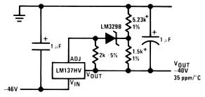
\*Use resistors with good tracking TC < 25 ppm/°C
