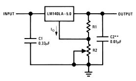
$V_{OUT} = 5V + (5V/R1 + I_O) R2$ 5V/R1 = 3 I<sub>O</sub> load regulation (L,) [(R1 + R2)/R1] (L, of LM140LA-5.0)
