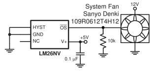
The fan's control pin has an internal pull-up. The 10 kOhm pull-down sets a slow fan speed. When the output of the LM26NV goes low, the fan will speed up.
