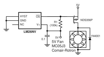
The LM26NV switches the fan on when the measured temperature exceeds the trip temperature.
