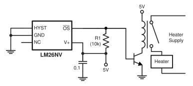
When the measured temperature is below the trip temperature of the LM26NV, the  $\overline{OS}$  output will be high, causing the switch and relay to close. When the temperature exceeds the trip point,  $\overline{OS}$  goes low and shuts off the relay and heater.
