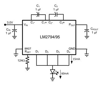
Figure 26. One Parallel Connected LED
