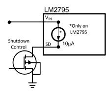
Figure 22. Open-Drain Logic Shutdown Control
