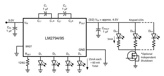
Figure 23. Keypad LEDs Connected to Pour
