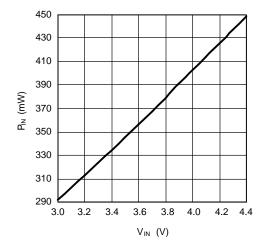
Figure 28.  $P_{IN}$  vs  $V_{IN}$  4 LEDs,  $2.5 \le V_{DX} \le 3.9V$ ,  $I_{DX} = 15mA$
