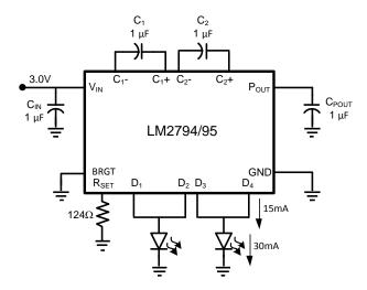
Figure 25. Two Parallel Connected LEDs
