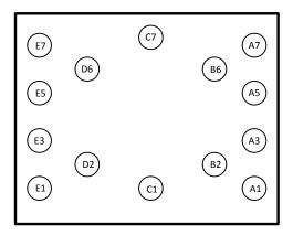
Figure 1. DSBGA Package Bottom View
