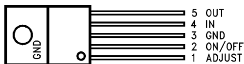
Figure 8. TO-220 5-Lead Power Package Front View
