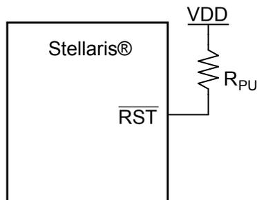
$R_{\text{PU}} = 0$  to 100 k $\Omega$
