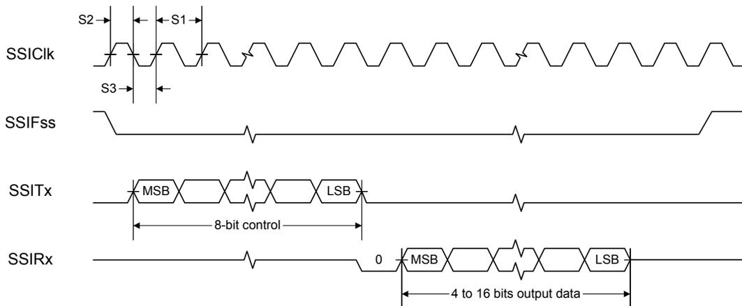
Figure 22-14. SSI Timing for SPI Frame Format (FRF=00), with SPH=1
