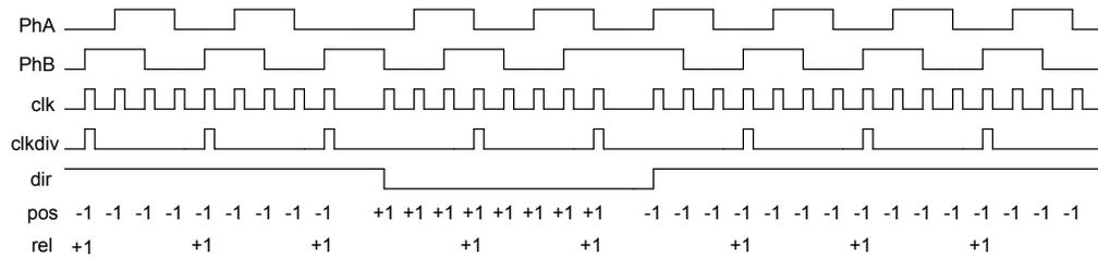
The period of the timer is configurable by specifying the load value for the timer in the **QELOAD** register. When the timer reaches zero, an interrupt can be triggered, and the hardware reloads the timer with the **QELOAD** value and continues to count down. At lower encoder speeds, a longer timer period is needed to be able to capture enough edges to have a meaningful result. At higher encoder speeds, both a shorter timer period and/or the velocity predivider can be used.
