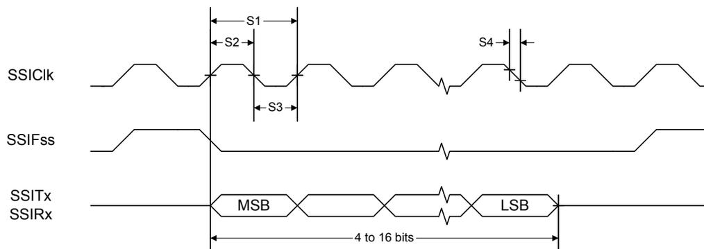
Figure 22-13. SSI Timing for MICROWIRE Frame Format (FRF=10), Single Transfer
