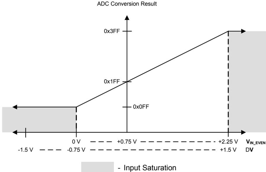
Figure 11-4. Differential Sampling Range,  $V_{IN\_ODD} = 2.25\text{ V}$
