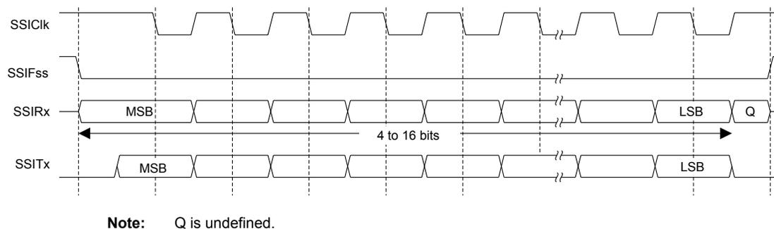
**Figure 13-8. Freescale SPI Frame Format (Continuous Transfer) with SPO=1 and SPH=0**
