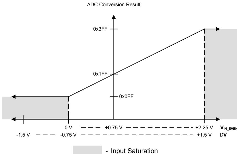
Figure 11-4. Differential Sampling Range,  $V_{IN\_ODD} = 2.25\text{ V}$
