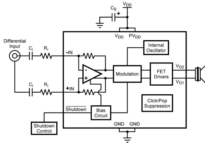
Figure 22. Differential Input Configuration with Input Capacitors
