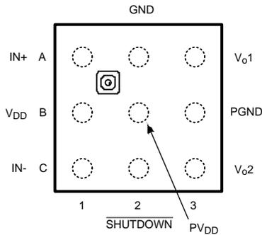
Figure 2. 9-Bump DSBGA - Top View
