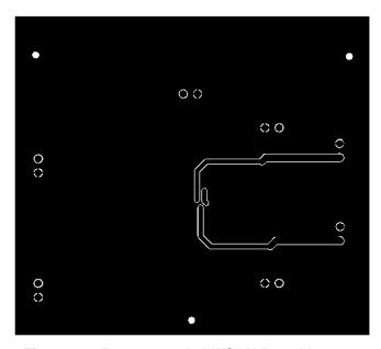
Figure 33. Recommended WSON Board Layout: Bottom Layer
