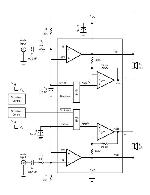
Figure 1. Typical Audio Amplifier Application Circuit
