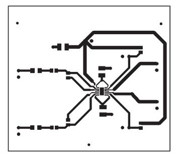
Figure 32. Recommended WSON Board Layout: Top Layer
