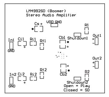
Figure 31. Recommended WSON Board Layout: Top Overlay
