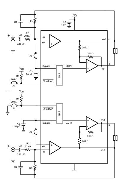
Figure 30. Higher Gain Schematic Drawing
