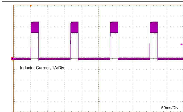
Figure 8-5. Inductor Current Burst in Short-Circuit Mode
