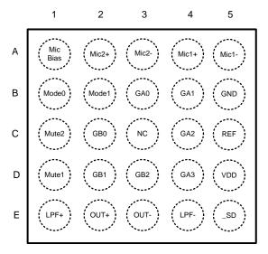
Figure 2. 25-Bump DSBGA (Top View) See YFQ0025 Package
