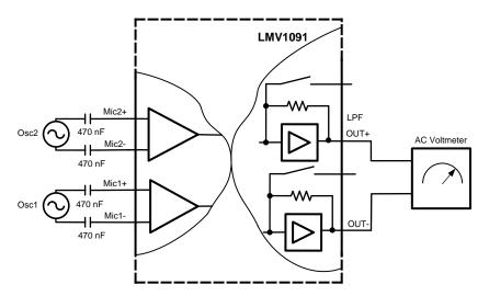
Figure 3. FFNS<sub>E</sub>, NFSL<sub>E</sub>, SNRI<sub>E</sub> Test Circuit
