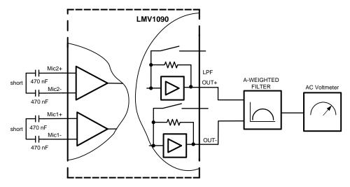
Figure 4. Noise Measurement Setup
