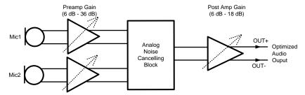
Figure 18. Simplified Block Diagram of the LMV1091
