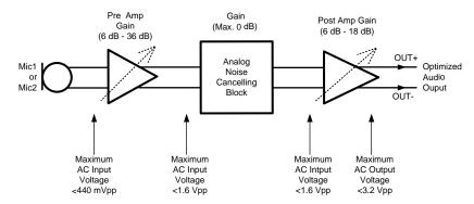
Figure 19. Maximum Signal Levels
