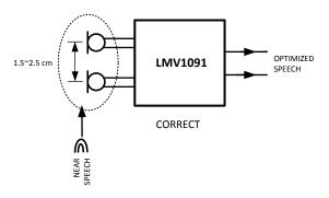
Figure 21. Endfire Array (CORRECT)
