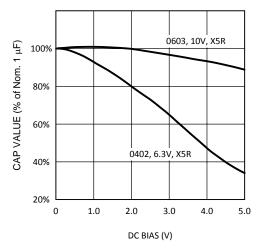
Figure 1. Capacitance versus DC Bias Plot
