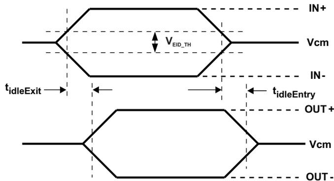
Figure 2. Electrical Idle Mode Exit and Entry Delay
