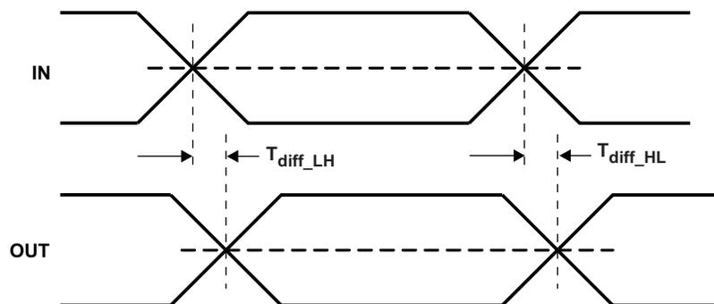
**Figure 1. Propagation Delay**
