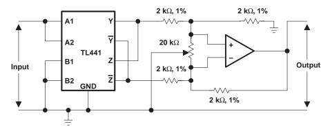
Figure 13. Utilization of Paralleled Inputs
