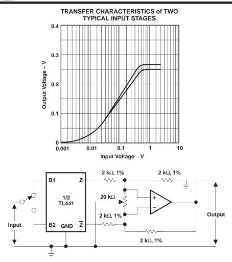
Figure 12. Utilization of Separate Stages
