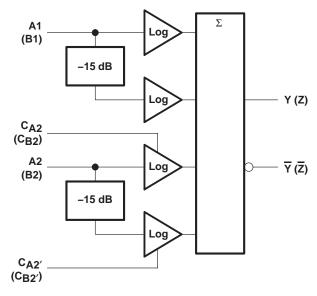
$Y \propto log~A1 + log~A2; Z \propto log~B1 + log~B2$  where: A1, A2, B1, and B2 are in dBV, 0 dBV = 1 V.  $C_{A2}, C_{A2'}, C_{B2}$ , and  $C_{B2'}$  are detector compensation inputs.
