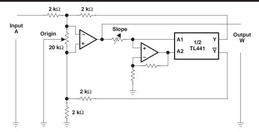
NOTE: Adjust the slope to correspond to the base "a". Exponential to any base: W = a.
