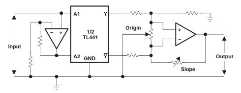
Figure 11. Output Slope and Origin Adjustment
