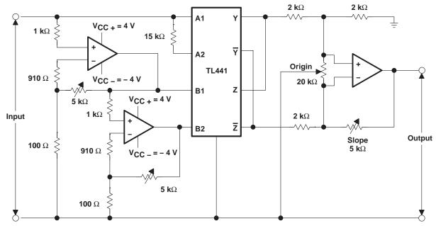
NOTES: A. nputs are limited by reducing the supply voltages for the input amplifiers to  $\pm 4~\text{V}.$
