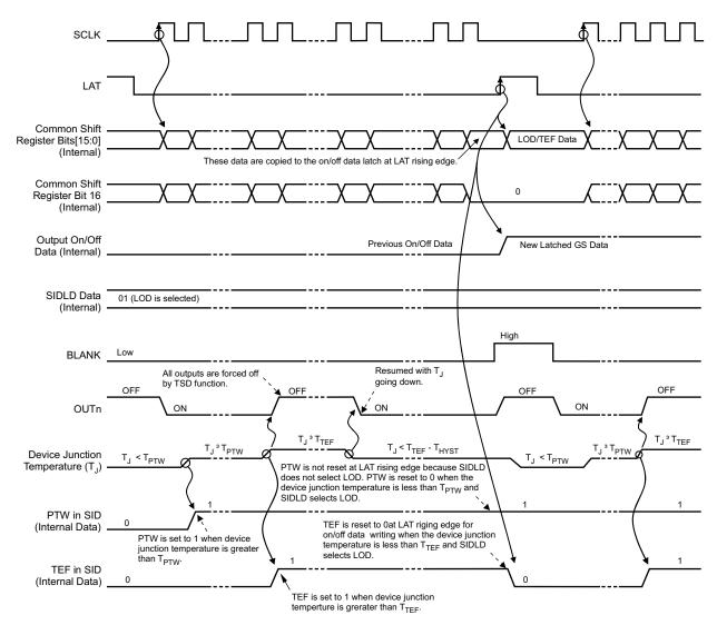
Figure 6. PTW/TEF/TSD Timing (LOD Selected)
