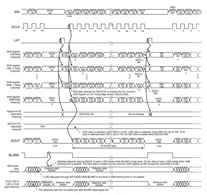
Figure 10. SID Read Timing
