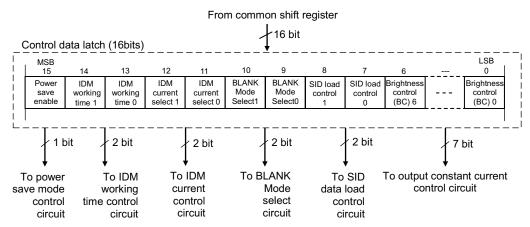
Figure 34. Function Control Data Latch Configuration
