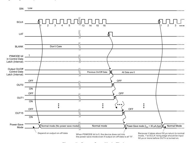
Figure 7. Power-Save Mode Timing
