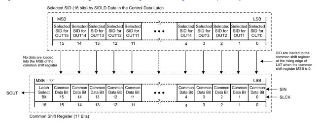
Figure 30. SID Load Configuration
