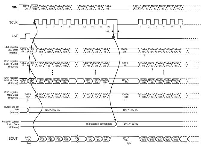
Figure 13. Function Control Data Write Timing
