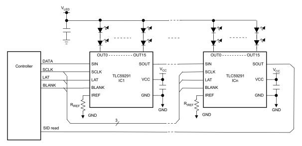
Figure 36. Multiple Daisy-chained TLC59291 Devices
