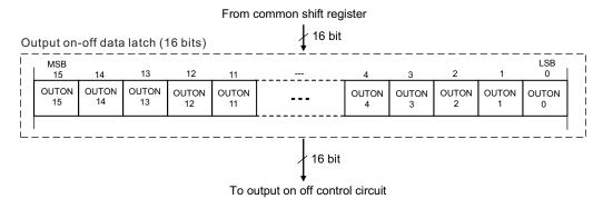
Figure 32. Output On/Off Data Latch Configuration
