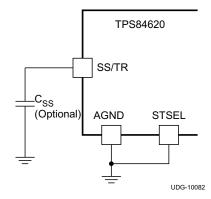
Figure 33. Slow-Start Capacitor (C<sub>SS</sub>) and STSEL Connection
