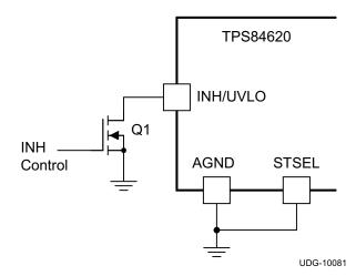
Figure 30. Typical Inhibit Control
