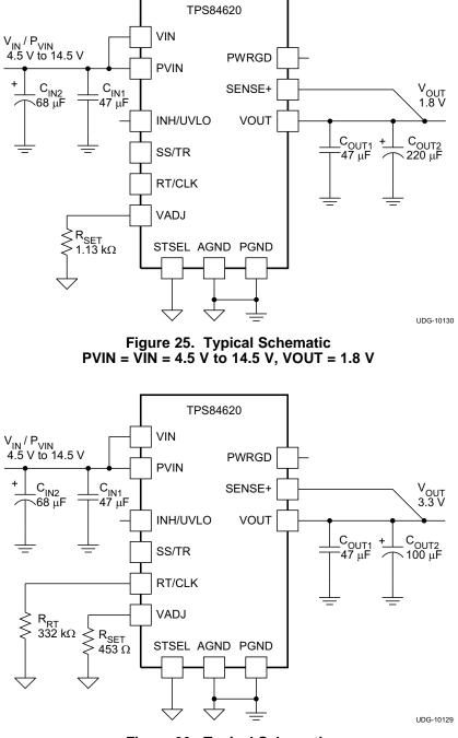
Figure 26. Typical Schematic PVIN = VIN = 4.5 V to 14.5 V, VOUT = 3.3 V
