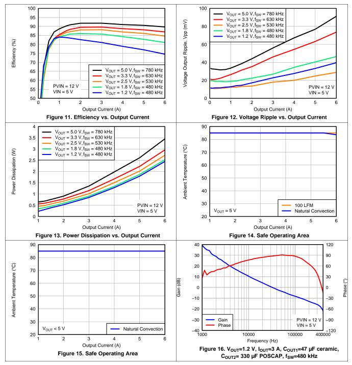
(1) The electrical characteristic data has been developed from actual products tested at 25°C. This data is considered typical for the converter. Applies to Figure 11, Figure 12, and Figure 13.
