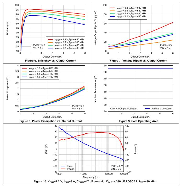
(1) The electrical characteristic data has been developed from actual products tested at 25°C. This data is considered typical for the converter. Applies to Figure 6, Figure 7, and Figure 8.
