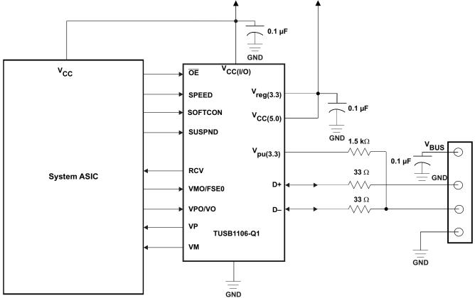
Figure 9. Peripheral-Side (Low-Speed) Regulator Bypass Mode
