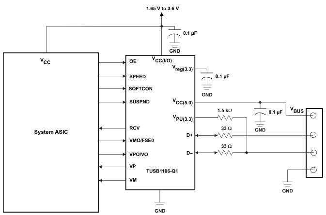
Figure 11. Peripheral-Side (Low-Speed) Internal Regulator Mode
