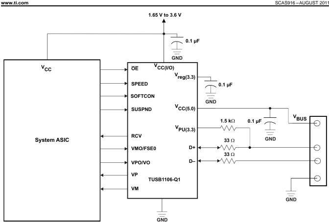
Figure 10. Peripheral-Side (Full-Speed) Internal Regulator Mode
