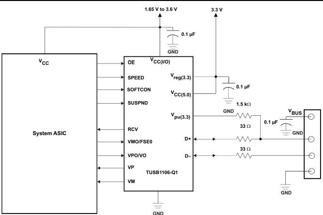
Figure 8. Peripheral-Side (Full-Speed) Regulator Bypass Mode
