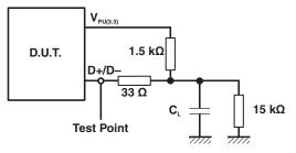
Figure 7. Load for D+, D-
