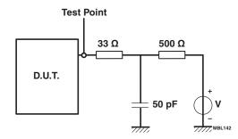
Figure 5. Load for Enable and Disable Times
