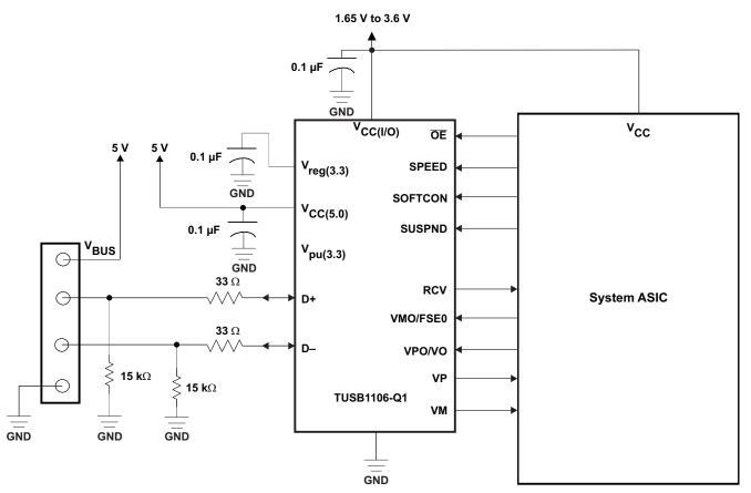
Figure 12. Host Side (V<sub>CC(5.0)</sub> Supplied From V<sub>BUS</sub> Pin)
