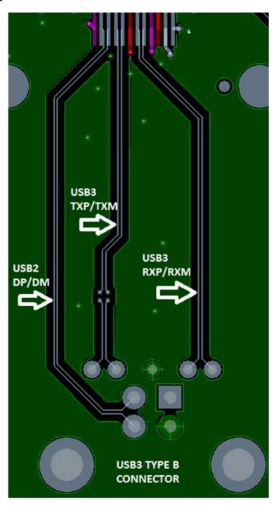
Figure 56. Example Routing of Upstream Port
