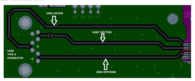
Figure 57. Example Routing of Downstream Port
