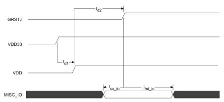
Figure 1. Power-Up Timing Requirements
