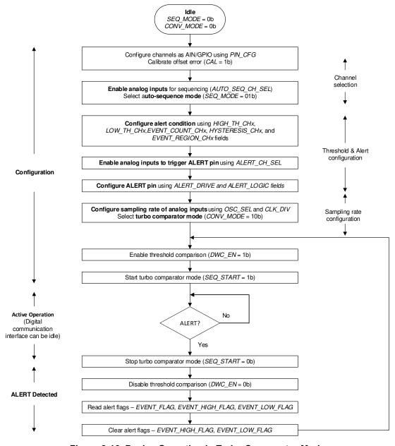
Figure 8-16. Device Operation in Turbo Comparator Mode
