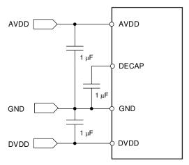
Figure 10-1. Power-Supply Decoupling
