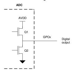
Figure 9-5. Digital Push-Pull Output
