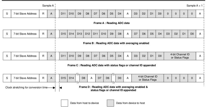
Figure 8-7. Data Frames for Reading Data
