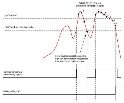
Figure 8-10. False Trigger Avoidance Using the Event Counter
