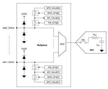
Figure 8-1. Analog Inputs, GPIOs, and ADC Connections
