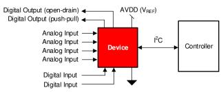
Figure 9-1. DAQ Circuit: Single-Supply DAQ
