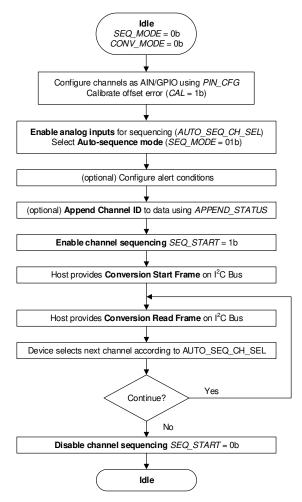
Figure 8-14. Device Operation in Auto-Sequence Mode
