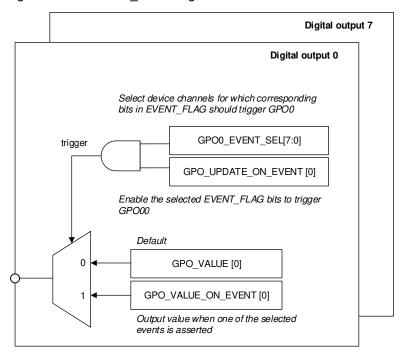
Figure 8-11. Block Diagram of the Digital Output Logic
