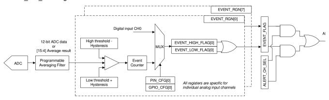
Figure 8-8. Digital Window Comparator Block Diagram
