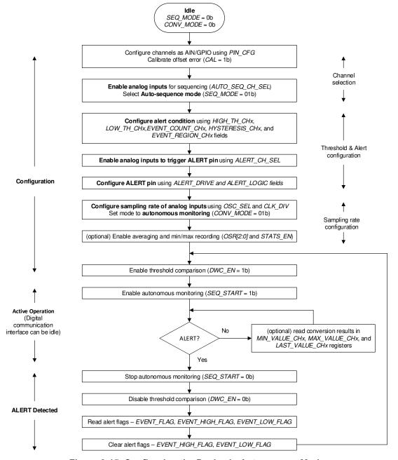
Figure 8-15. Configuring the Device in Autonomous Mode
