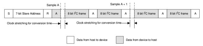
Figure 8-13. Starting a Conversion and Reading Data in Manual Mode
