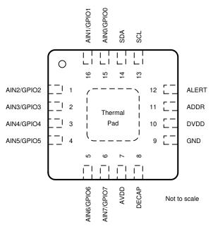
Figure 6-1. RTE Package, 16-Pin WQFN, Top View
