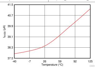
Figure 7-24. Analog Supply Current vs Temperature (OSC\_SEL = 1, CLK\_DIV = 0) in Turbo Comparator Mode
