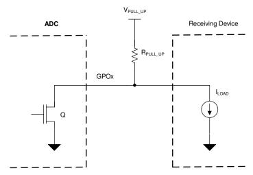
Figure 9-3. Digital Open-Drain Output
