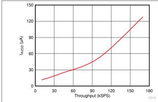
Figure 7-20. Analog Supply Current vs Throughput
