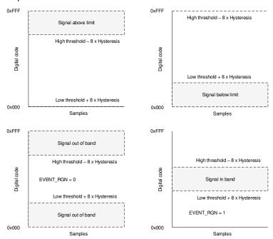
Figure 8-9. Event Monitoring With the Window Comparator
