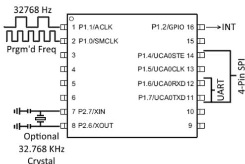
**Figure 1. Programmable Clock Source I/Os**
