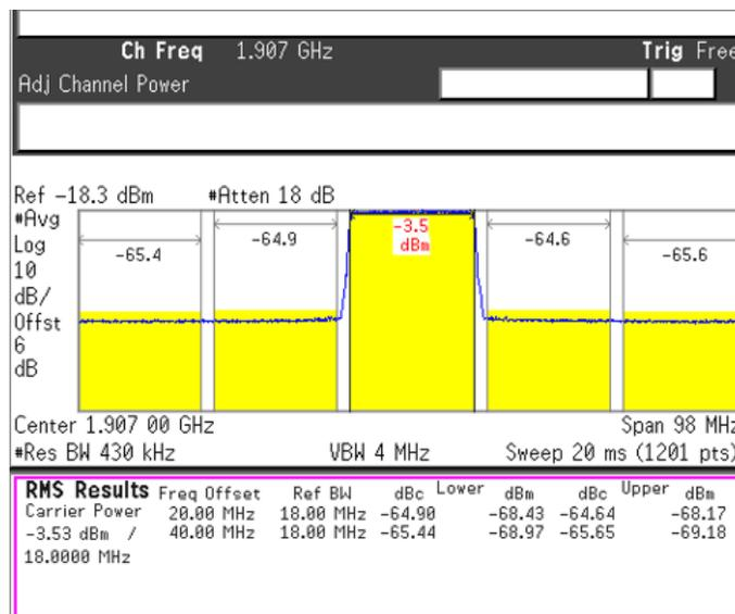
Figure 9. Repeater ACPR Measurement From Output Shows 6-dB Gain of Waveform and 8-dB ACPR Degradation
