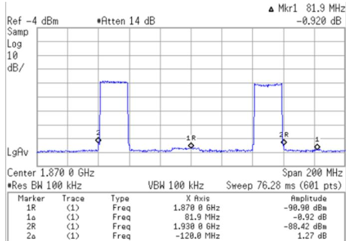
Figure 11. Repeated Wideband Signal Simulating a 120-MHz Carrier
