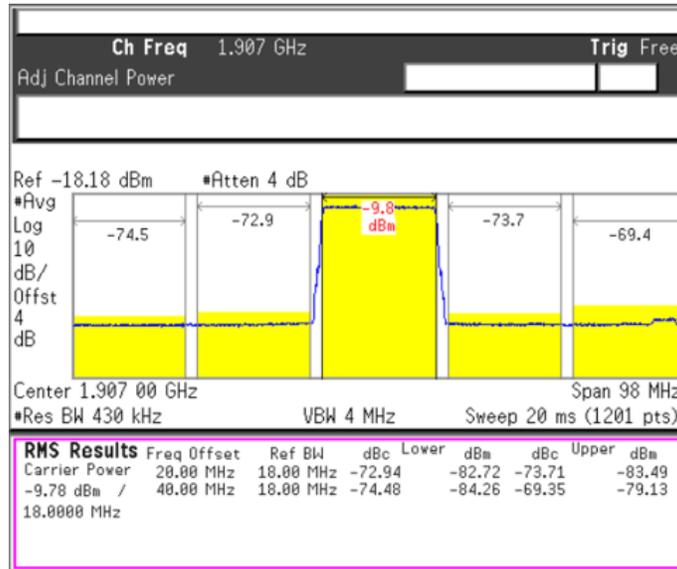
Figure 8. Clean ACPR Measurement Directly From DAC38RF82
