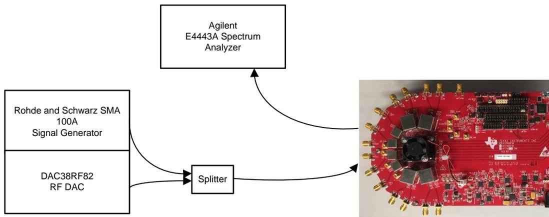
**Figure 10. Hardware Setup for Jammer Simulation**
