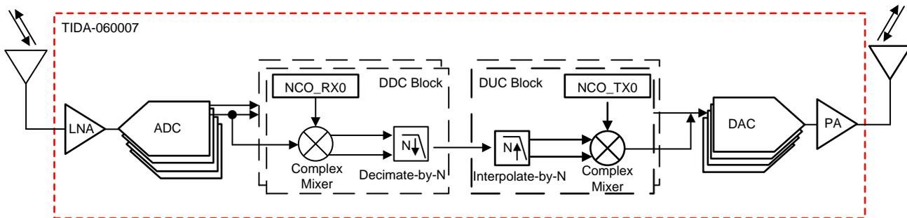
Figure 2. TIDA-060007 Block Diagram
