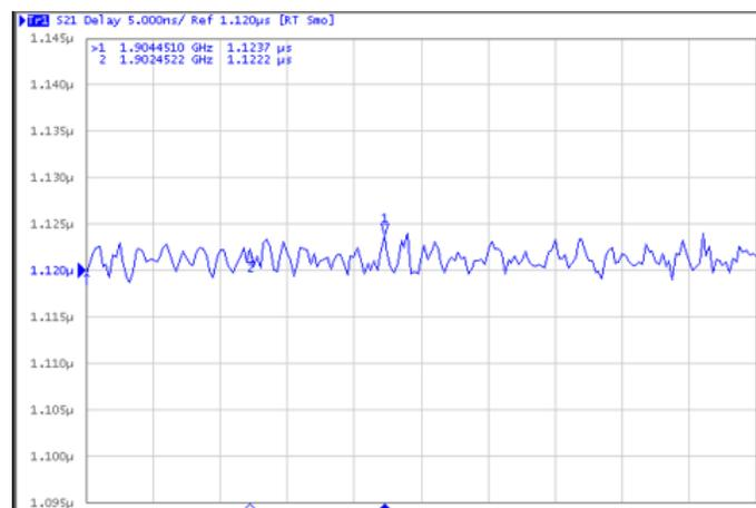
Figure 5. Latency Measurement, Average Latency = 1.12  $\mu$ s
