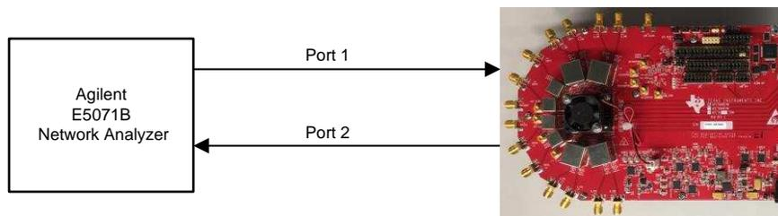
Figure 4. Latency and Gain Test Setup
