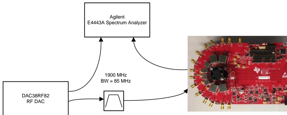
Figure 7. Test Setup for ACPR Degradation
