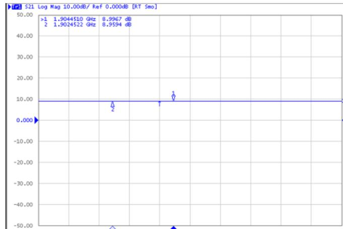
Figure 6. Gain Measurement: Gain is Flat at 9 dBm With TX/RX DSA set to 0
