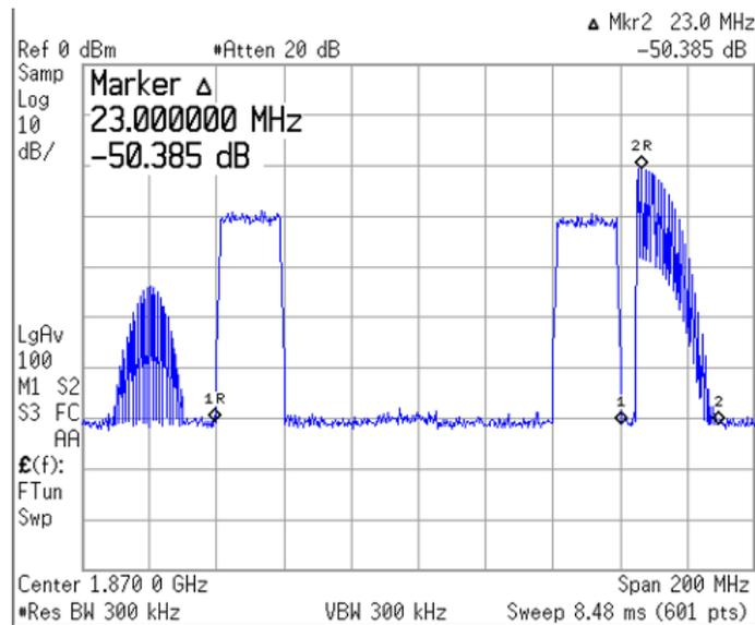
Figure 12.  $-50$ -dBc Attenuation at 23-MHz Outside Decimation Bandwidth
