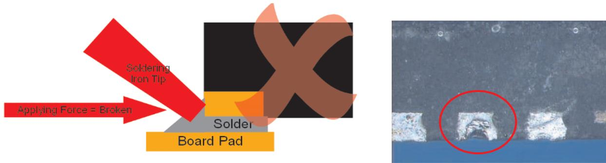
**Figure 18. Manual Rework Damage**
