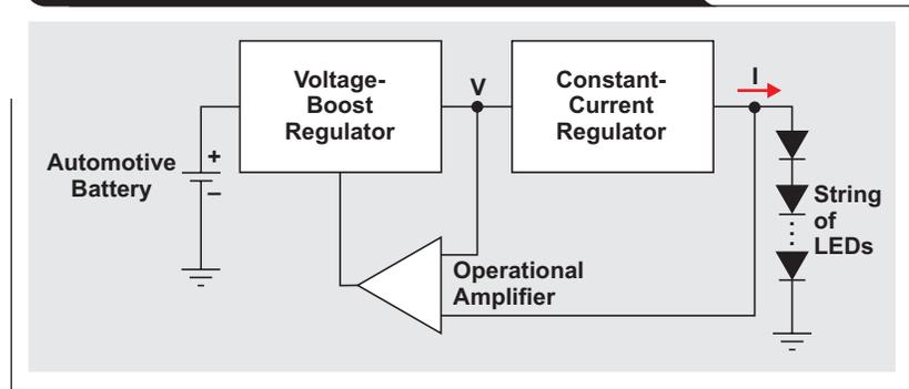
the worst-case LED string voltage and the worst-case dropout voltage of the linear constant-current regulator, which is assumed to be 1 V. This approach to choosing the linear constant-current regulator voltage guarantees startup for all conditions. Using the LED and linear LED driver parameters in Table 1, the pre-boost voltage is 29 V, as given by Equation 2.
