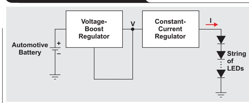
forward-voltage characteristics. If the number of LEDs changes by  $N$ , then the voltage at the output of the constant-current regulator changes by  $NV_F$ , where  $V_F$  is the forward voltage of each LED.
