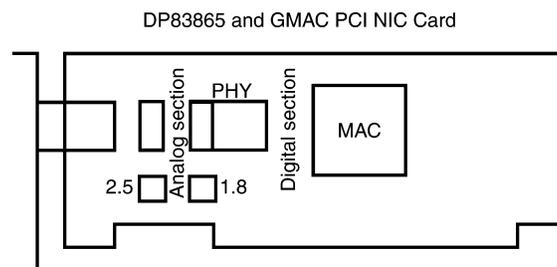
**Figure 4. 1.8 V Voltage Regualtor Placement**
