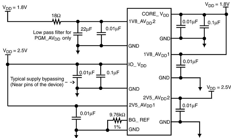
Figure 3. Power Supply Filtering (One Port)
