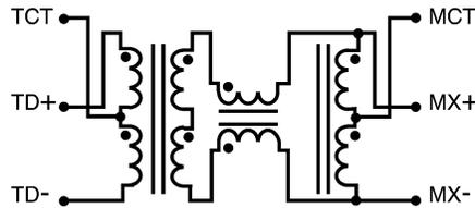
Figure 12. Transformer Configuration (1 ch)
