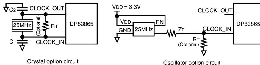
**Figure 1. Clock Input Circuit**
