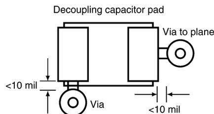
**Figure 2. Place Via Close to Pad**
