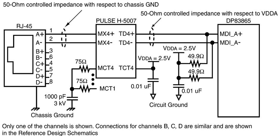
**Figure 8. Twisted Pair/Magnetics Interface (Channel A)**
