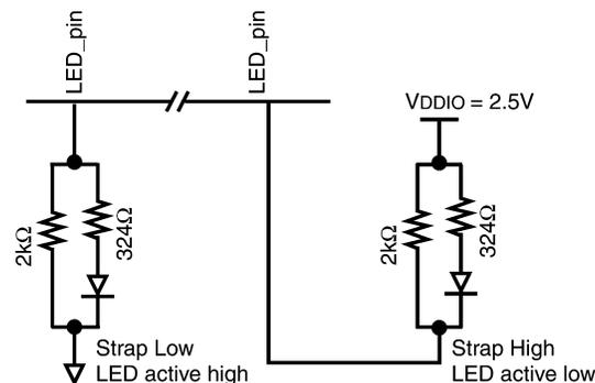
Figure 11. LED/Strapping Option examples
