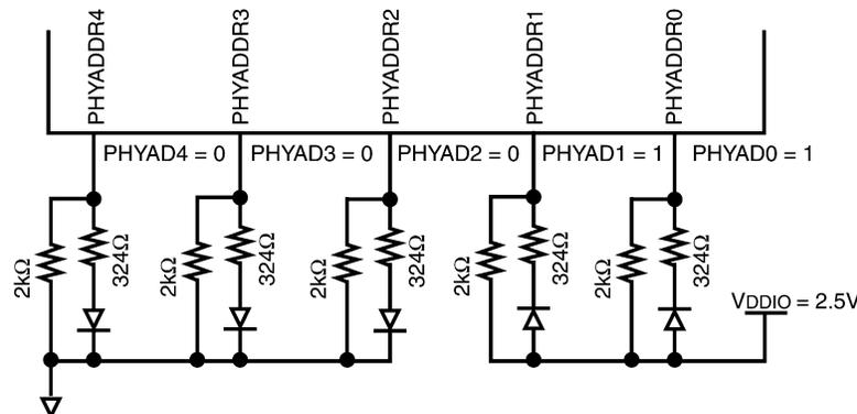
Figure 10. PHYAD/LED Strap Configuration. (PHY base address = 3)
