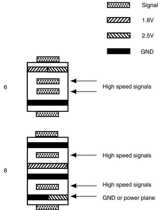
Figure 5. PCB Layer Stacking, Circuit Side
