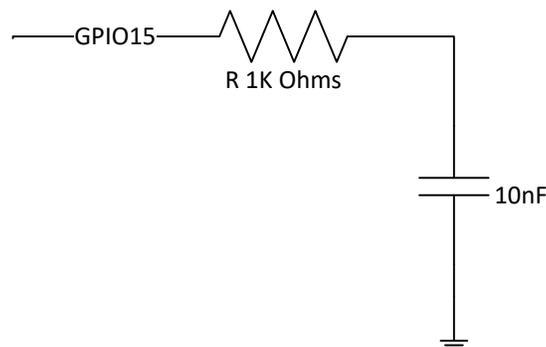
**Figure 1. Hardware Connections**
