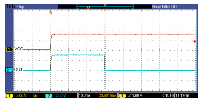
Figure 14. TMP303A Power-On Response, T_A Less Than 60°C
