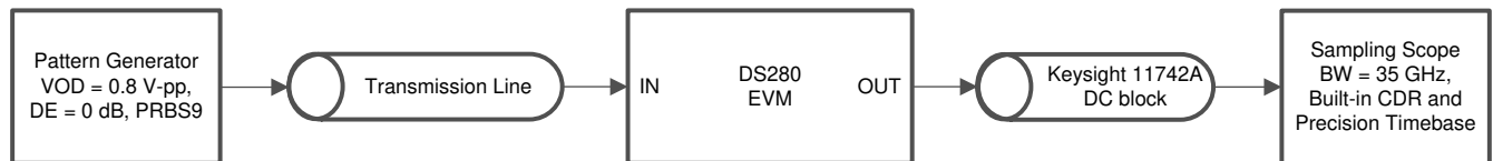
図 9-13. 5 in input channel and minimal output channel test setup
