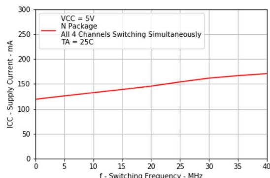
[図 5-1. Supply Current vs Switching Frequency](#)
